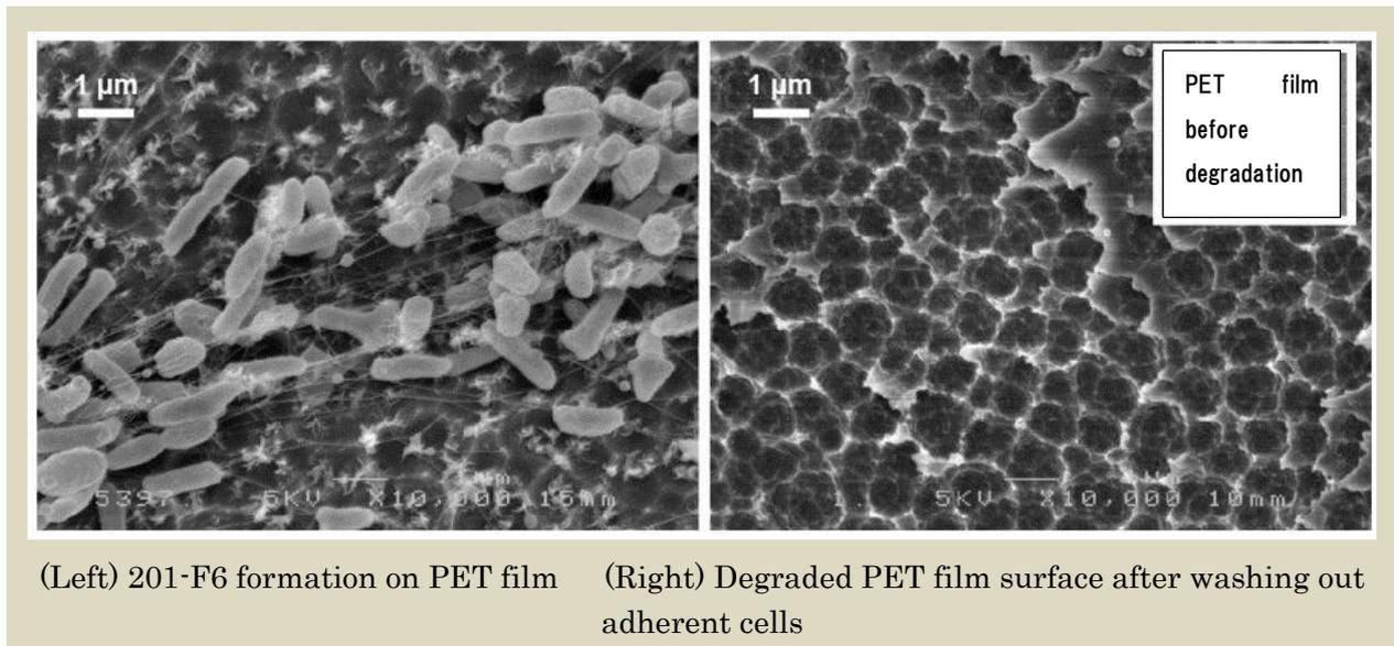
(Left) 201-F6 formation on PET film (Right) Degraded PET film surface after washing out adherent cells
